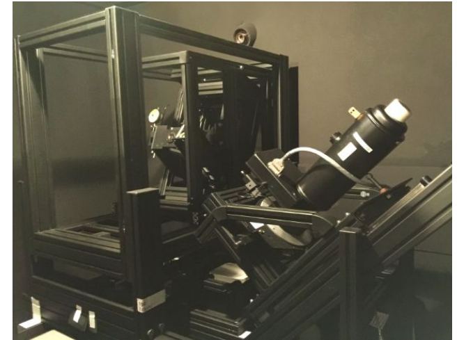
Echelle grating, crossdisperser and the detector
